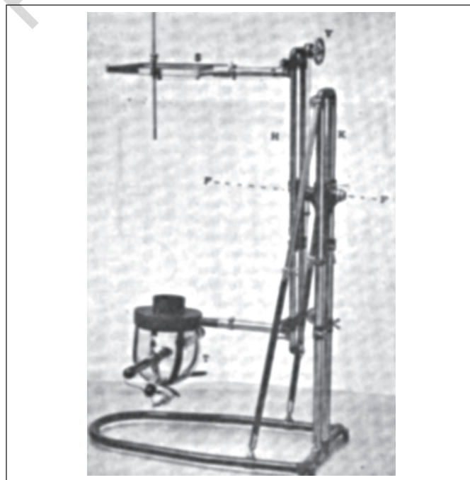
Fig. 4: The Baese’s portable Radiostereometre: the X-rays emitting tube and the plate holder are joined and the entire apparatus can be moved, rotated or spiralled so as to obtain rapid double exposures. It anticipated the concept of stratigraphy and CT scanning [31]
